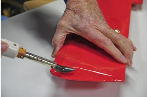
Trim off the excess covering, and seal it in place with the covering iron. Using the trim iron, shrink the covering staying away from the seams on both sides. Gently glide the iron over the surface until the covering is wrinkle-free. You will have to do this four times, on each side of each tip, to complete the wing.
